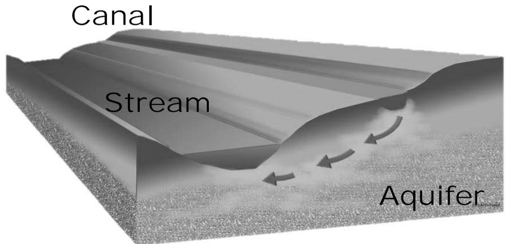
Conjunctive Water Management is an *adaptive process* that utilizes the *connection* between surface water and groundwater to *maximize water use*, while *minimizing impacts* to streamflow and groundwater levels in an effort to increase the overall water supply of a region and improve the reliability of that supply.
