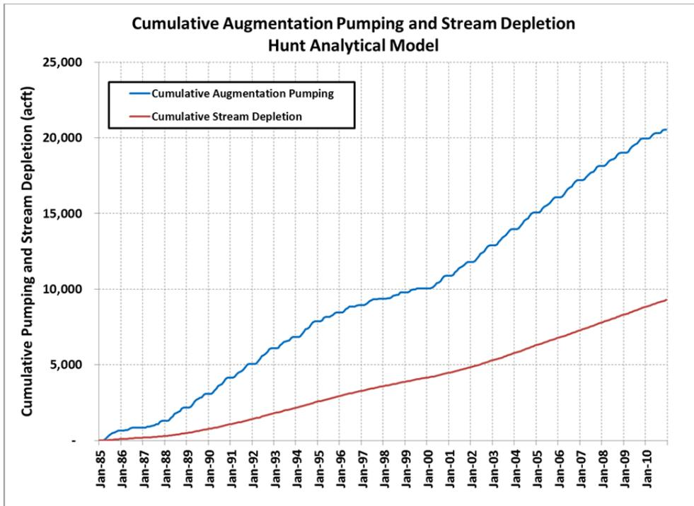
**Figure 5-2: Cumulative Augmentation Well Pumping and Stream Depletion for 26-year Scenario with Hunt Analytical Model**
