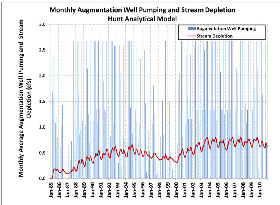
**Figure 5-1: Monthly Augmentation Well Pumping and Stream Depletion for 26-year Scenario with Hunt Analytical Model**
