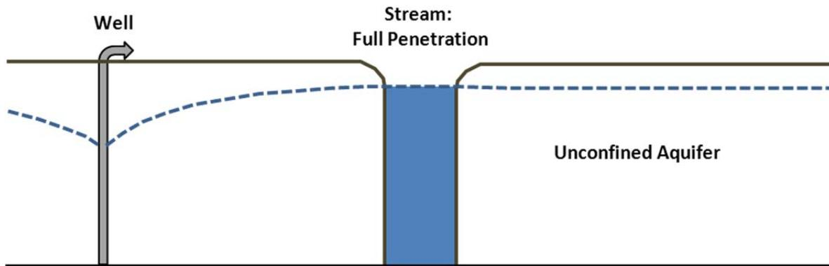
Figure 3-1a: Conceptual Model with Fully Penetrating Stream (Glover and Balmer 1954)
