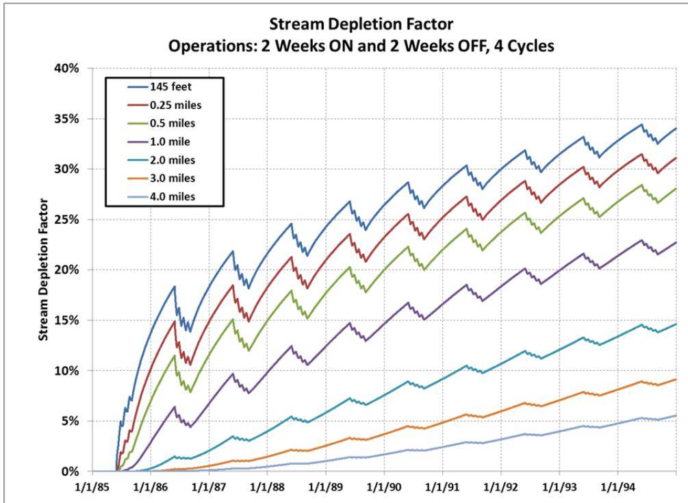
Figure 8-6: Stream Depletion Factors for 2 Weeks On and 2 Weeks Off Operations with Well at Various Distances from Stream
