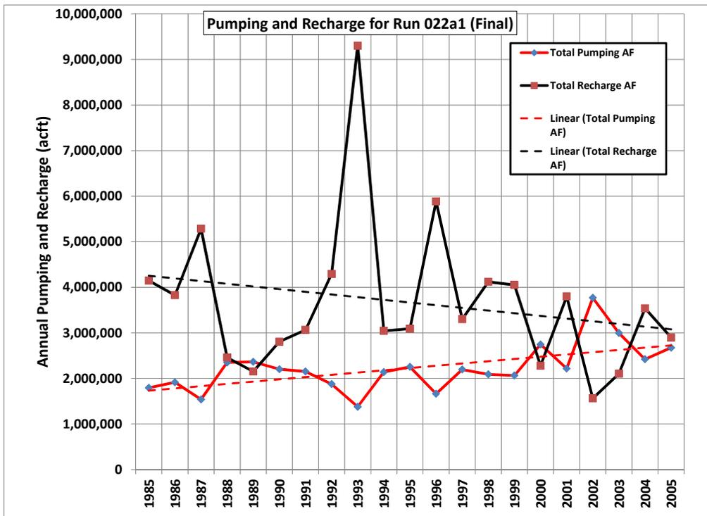
Figure 4-2: Annual Pumping and Recharge in Draft COHYST 2010 Groundwater Model
