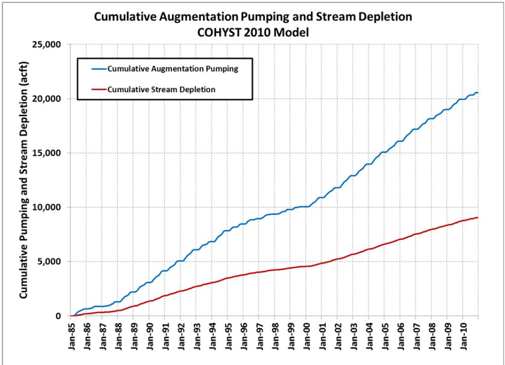
**Figure 5-5: Cumulative Augmentation Well Pumping and Stream Depletion for 26-year Scenario with COHYST 2010 Model**
