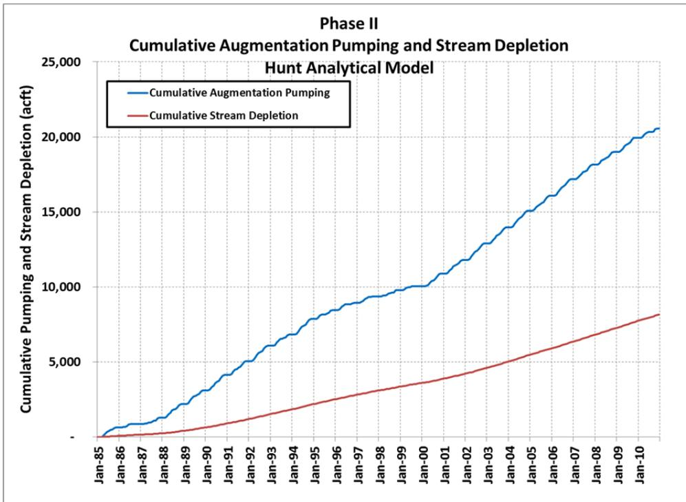
Figure 9-3: Phase II Augmentation Well - Cumulative Augmentation Well Pumping and Stream Depletion for 26-year Scenario with Hunt Analytical Model
