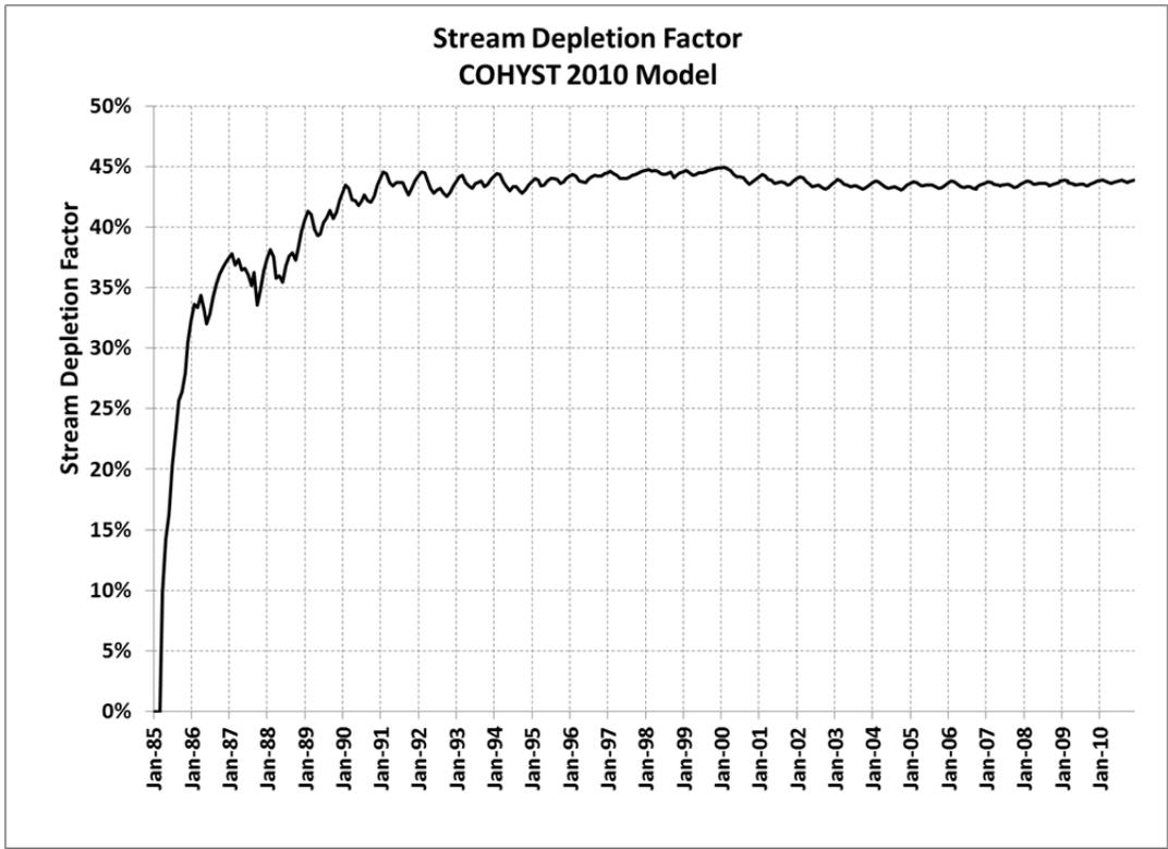
**Figure 5-6: Stream Depletion Factor for 26-year Scenario with COHYST 2010 Model**
