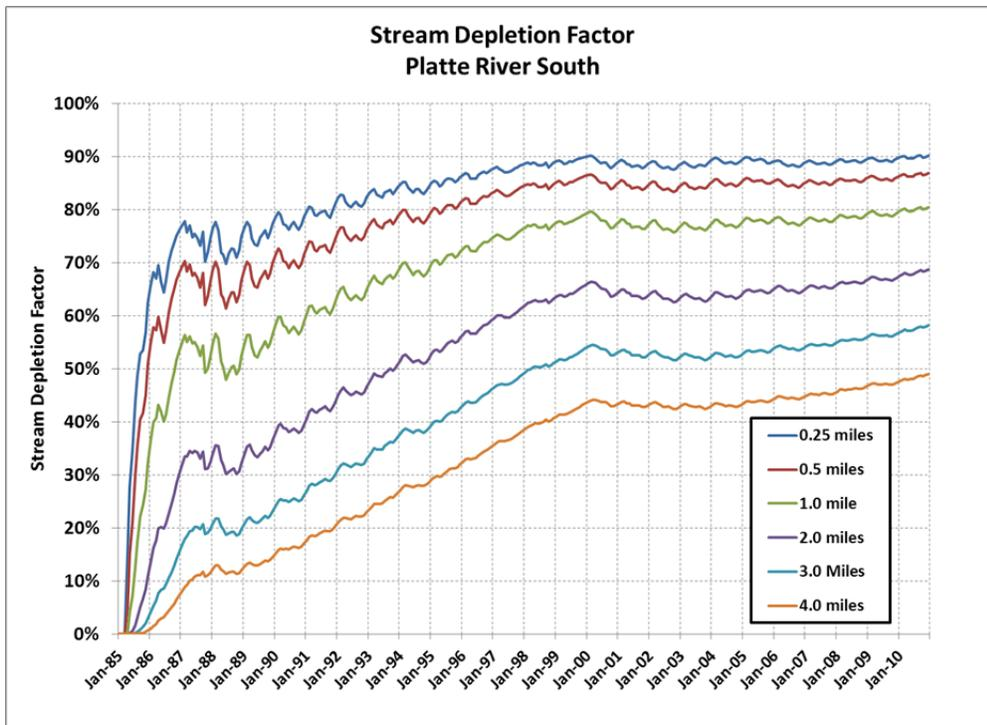
Figure 7-2: Stream Depletion Factor for Sensitivity Test with Augmentation Well at Various Distances from Platte River South
