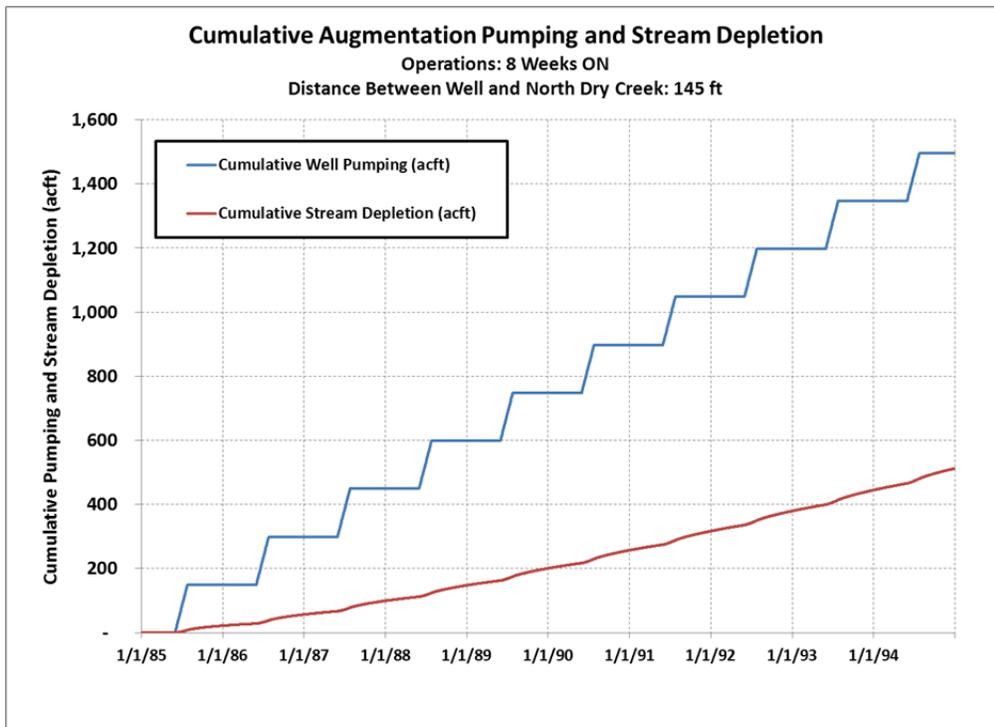
**Figure 8-2: Cumulative Augmentation Well Pumping and Cumulative Stream Depletion for 8 Weeks of Continual Operation**
