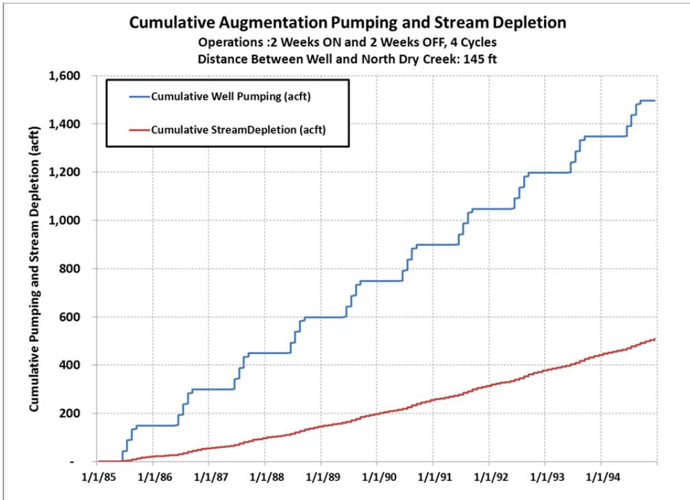
**Figure 8-5: Cumulative Augmentation Well Pumping and Cumulative Stream Depletion for 2 Weeks On and 2 Weeks Off Operations**
