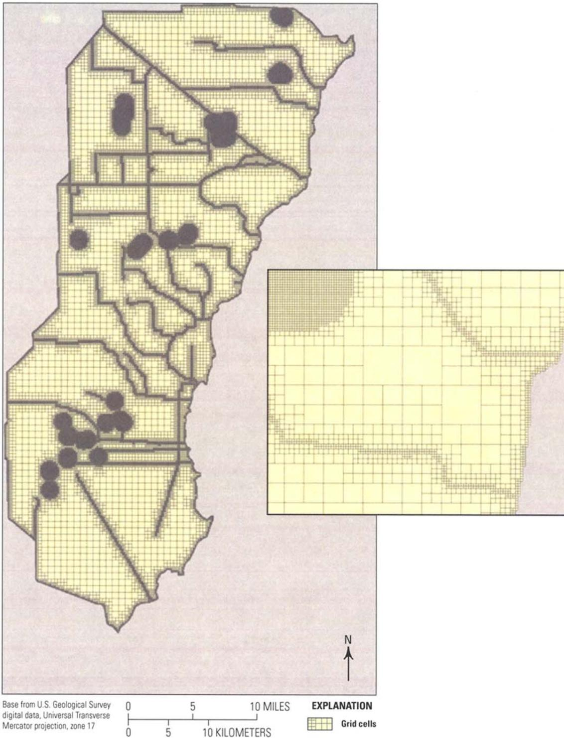
**Figure 3-4: Example of a MODFLOW Model using Structured and Unstructured Grids**
