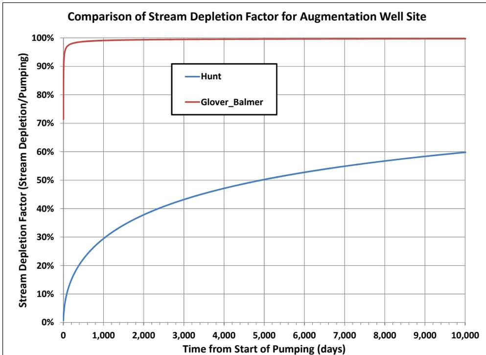
Figure 4-1: Comparison of Stream Depletion Factors with Glover-Balmer and Hunt Methods for North Dry Creek Site
