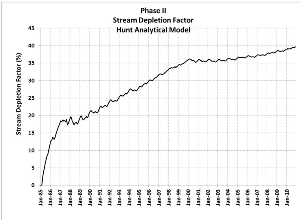
Figure 9-4: Phase II Augmentation Well - Stream Depletion Factor for 26-year Scenario with Hunt Analytical Model
