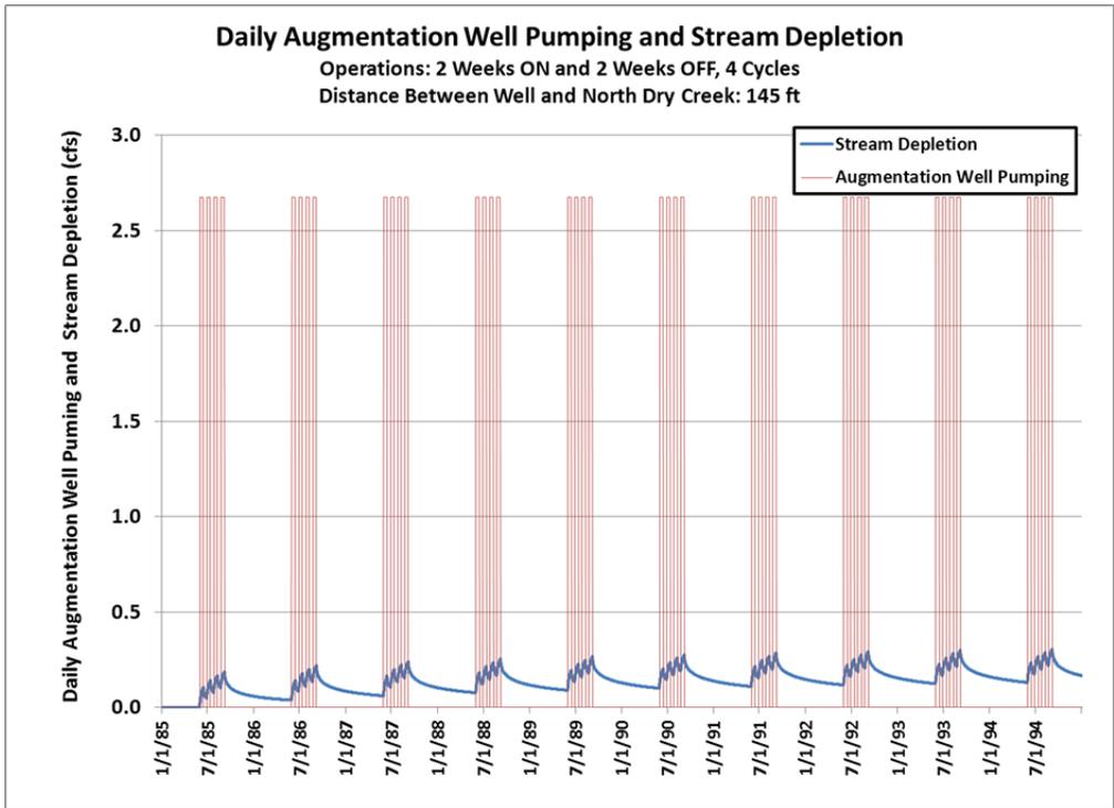
**Figure 8-4: Augmentation Well Pumping and Stream Depletion Factor for 2 Weeks On and 2 Weeks Off Operations**
