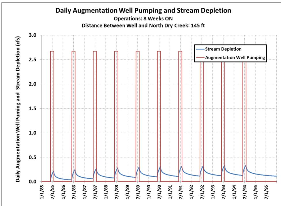
Figure 8-1: Augmentation Well Pumping and Stream Depletion Factor for 8 Weeks of Continual Operations
