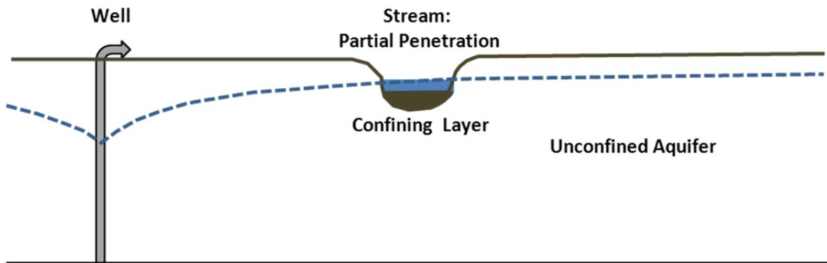
Figure 3-1b: Conceptual Model with Semipervious Streambed and Partial Penetrating Stream (Hunt 1999)
