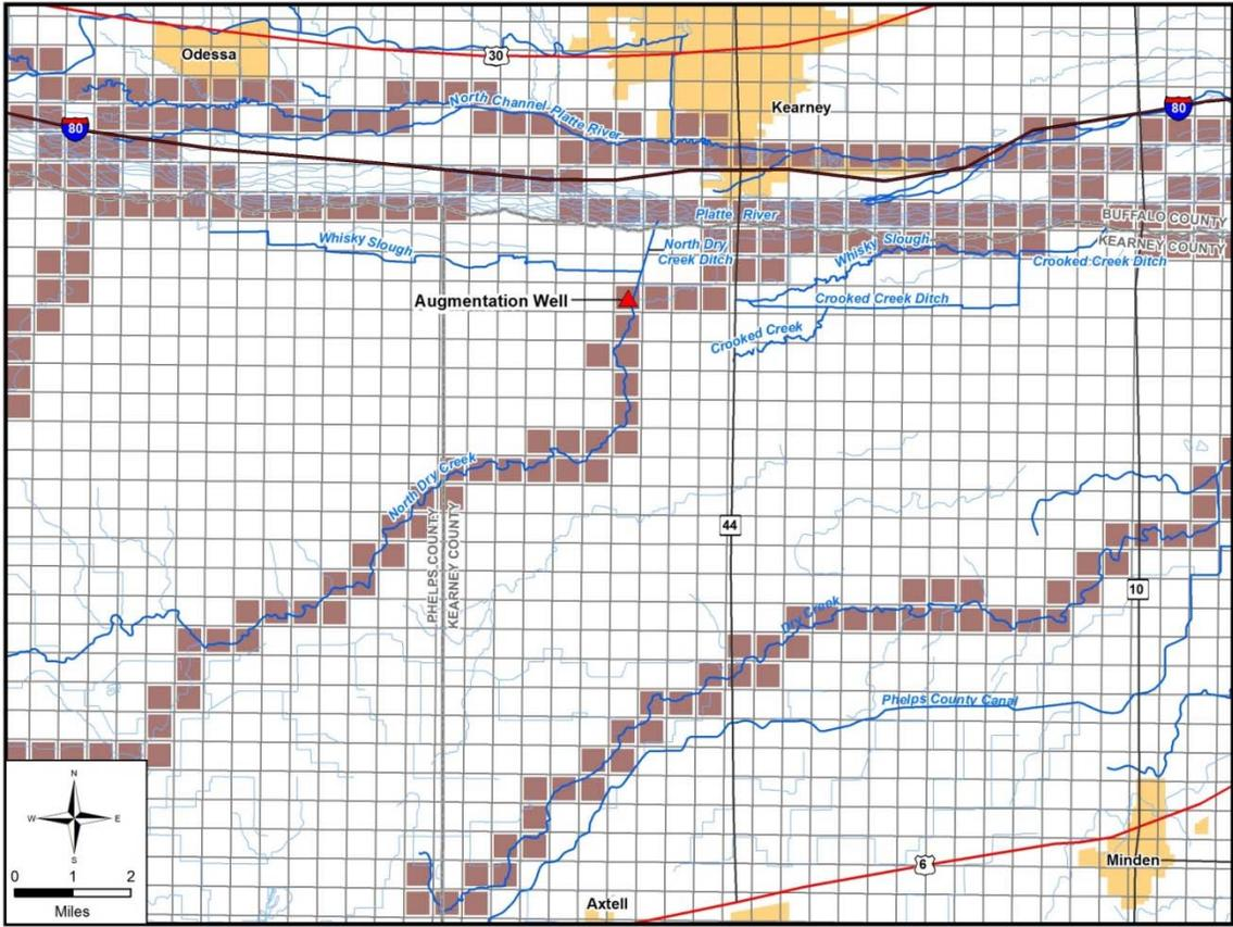
**Figure 3-2: Map Showing COHYST 2010 Groundwater Model Grid and Stream Cells**
