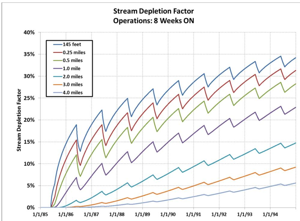
**Figure 8-3: Stream Depletion Factors for 8 Weeks of Continual Operations with Well at Various Distances from Stream**
