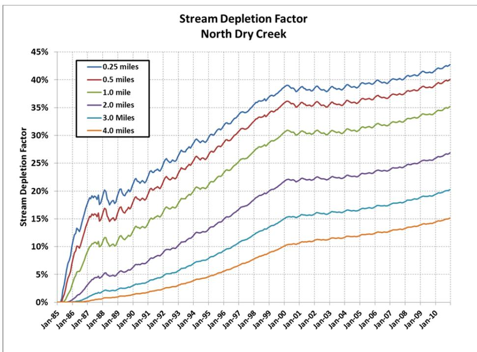
Figure 7-1: Stream Depletion Factor for Sensitivity Test of Augmentation Well at Various Distances from North Dry Creek
