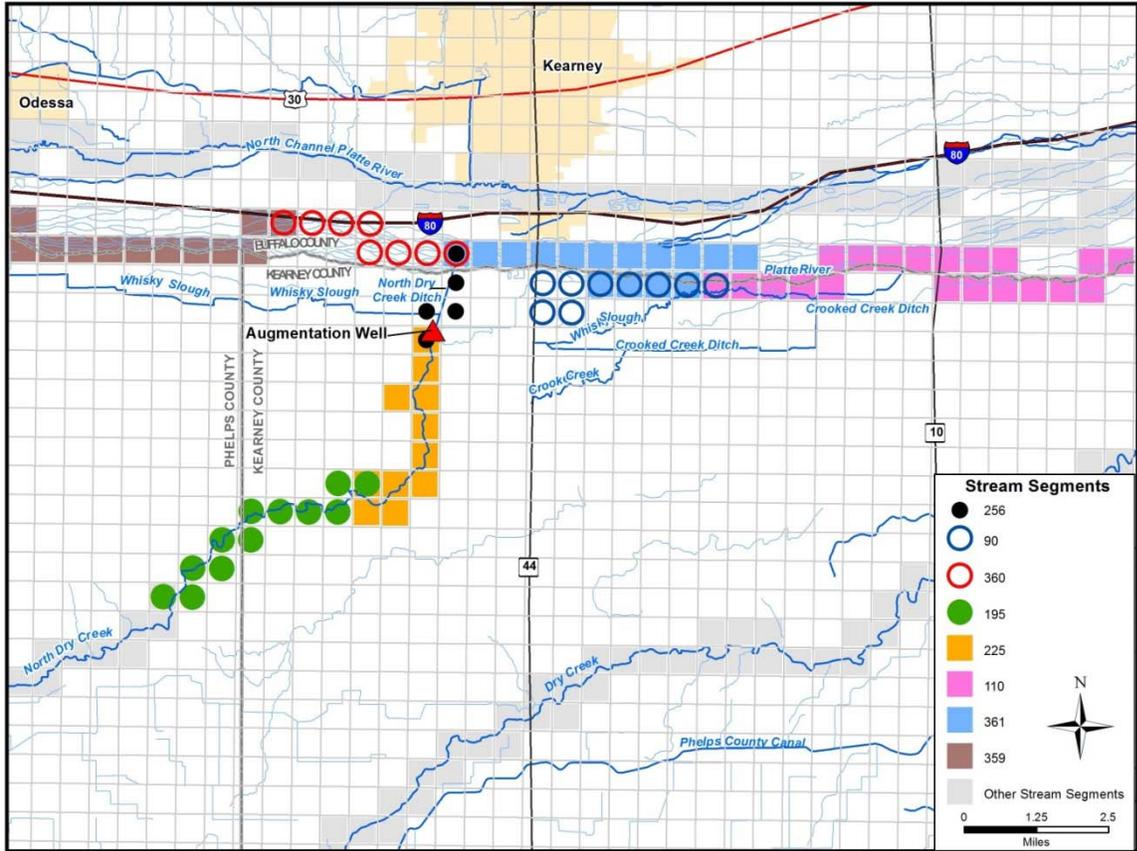
**Figure 4-3: MODFLOW Grid with Revised Stream Network on North Dry Creek and Locations of Stream Segments**
