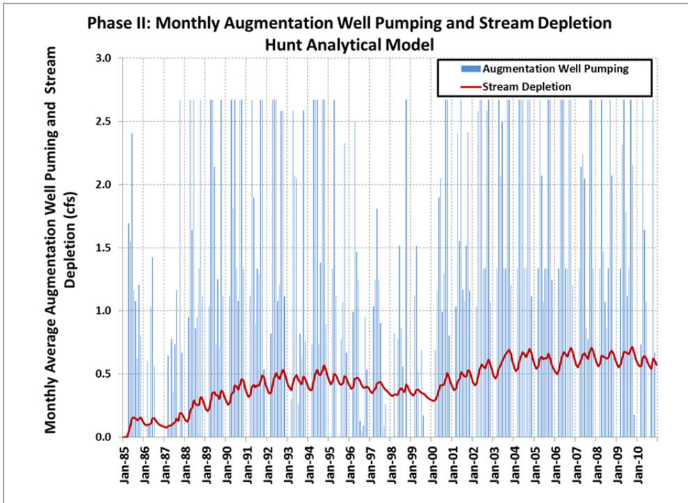
Figure 9-2: Phase II Augmentation Well - Monthly Augmentation Well Pumping and Stream Depletion for 26-year Scenario with Hunt Analytical Model
