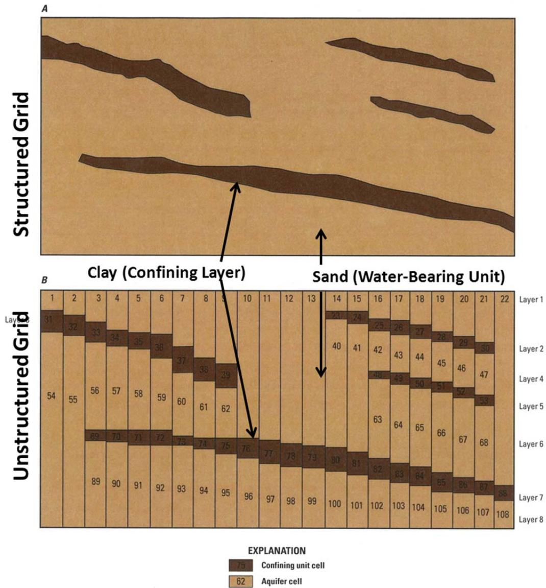
Figure 3-6: Comparison of Model Layer Discretization with Structured and Unstructured Grid
