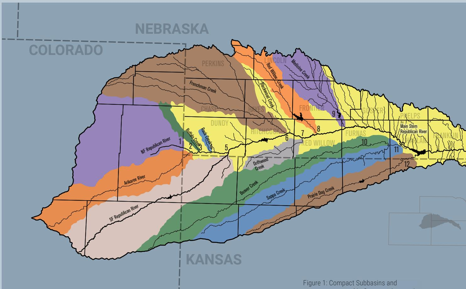
Figure 1: Compact Subbasins and streamgages used in Compact Accounting
