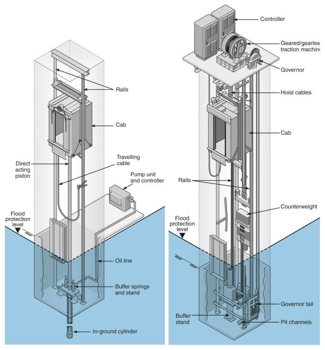
Figure 4-36. Typical elements of hydraulic elevators (left) and traction elevators (right). (Source: Otis Elevator Company).
