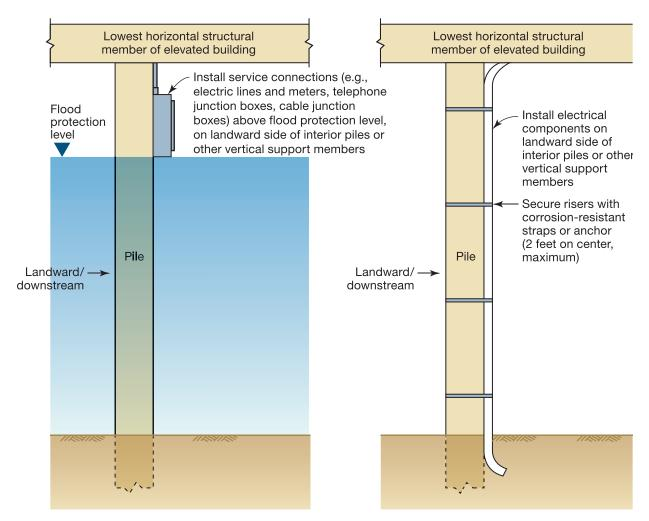
Figure 5-17. Placement recommendation for water meters exposed to moving floodwater.
