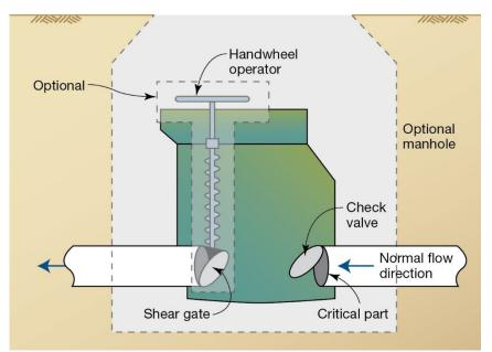
Figure 4-24. Combination gate and check valve.
