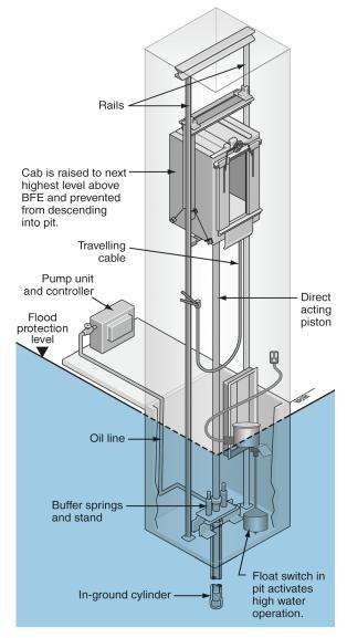
Figure 4-38. Float switch to control cab descent (Source: Otis Elevator Company).
