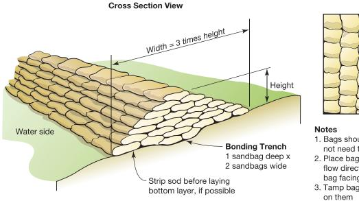
Figure 3-5. Techniques for proper placement of sandbags.
