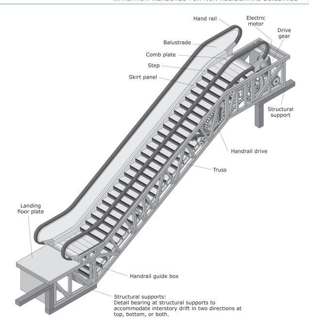
Figure 5-26. Typical elements of an escalator (Source: Otis Elevator Company).
