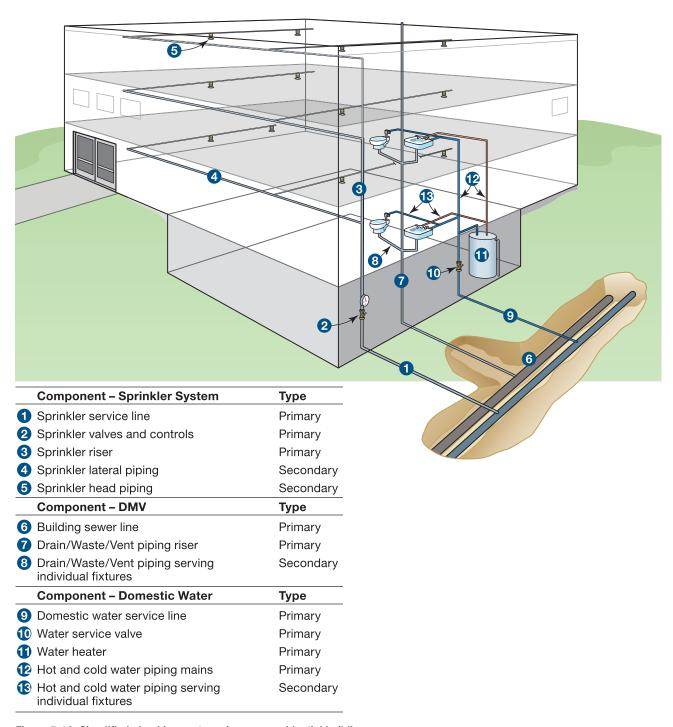
Figure 5-16. Simplified plumbing systems in a non-residential building.
