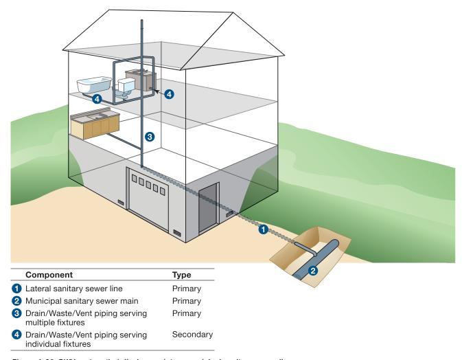
Figure 4-20. DWV system that discharges into a municipal sanitary sewer line.
