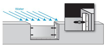
Figure 4-8. Alternate dry floodproofing methods for protecting equipment.
