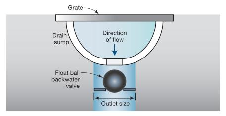
Figure 5-19. Floor drain with ball float check valve.
