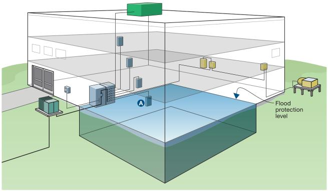
A Note: The basement panel will remain vulnerable to flooding. The panel should be electrically isolatable from the rest of the electrical system.
