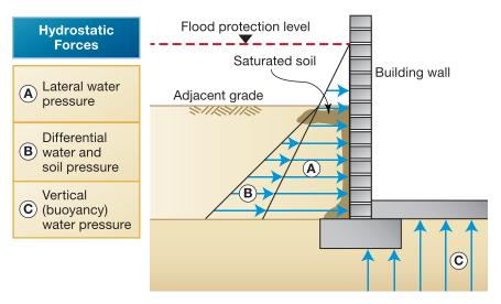
Figure 1-4. Hydrostatic forces.
