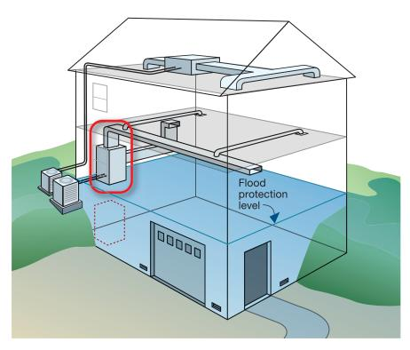
Figure 4-6. Relocating the basement HVAC unit to the first floor and placing exterior units at a higher grade provides greater flood protection than in-place elevation.
