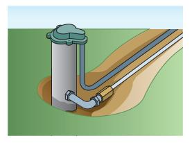
Figure 4-25. Sanitary well cap.
