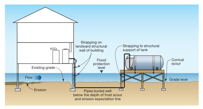
Figure 4-31. Protecting fuel piping from moving floodwater.
