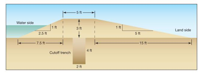
Figure 6-48. Valley House levee cross-sectional dimensions
