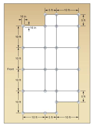
Figure 6-21. Timber pile plan for the elevated Chester house
