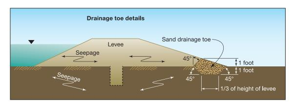
Figure 5F-29. Drainage toe details
