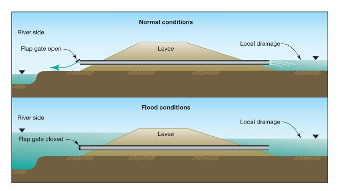
Figure 5F-30. Drain pipe extending through levee
