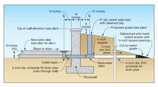
Figure 5F-21. Typical gravity floor drain
