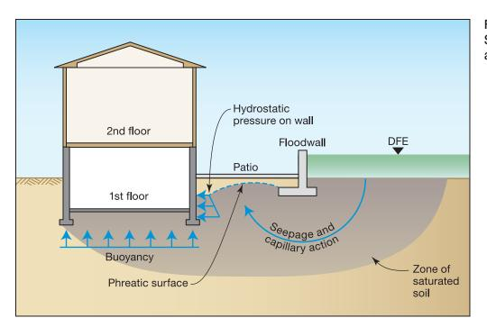
Figure 5F-9. Seepage underneath a floodwall
