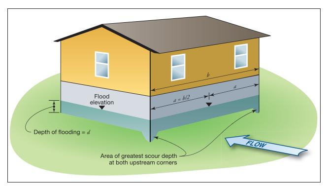
Figure 4-24. Scour action on a ground level building
