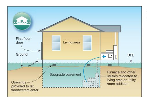
Figure 1-10. Wet floodproofed structure
