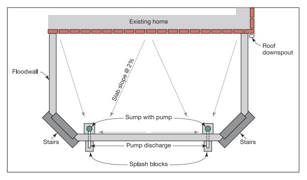
Figure 5F-20. Sample patio drainage to a sump
