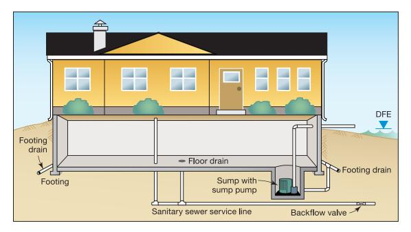
Figure 5D-8. Dry floodproofed homes should have an effective drainage system around footings and slabs to reduce water pressure on foundation walls and basements. The drainage systems can be extremely vulnerable to hydrostatic forces under high flooding conditions.
