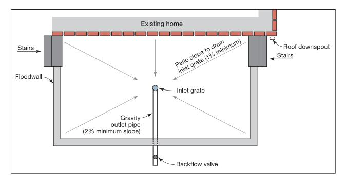
Figure 5F-19. Sample patio drainage to an outlet
