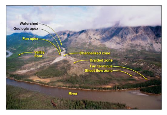
**Sheet Flow Zone:** Downstream of the braided zone characterized by flow depths less than ½ foot (flow depths normally decrease in the downfan direction). Smaller channels may aggrade while other areas are subject to erosion or scour. Flow may continue to spread laterally until sheet flow is predominant. Floods are usually limited to inundation by low velocity floodwater.
