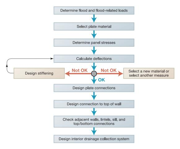
Figure 5D-21. Selection/design of plate shields
