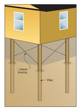
Figure 1-5. Elevation on piles
