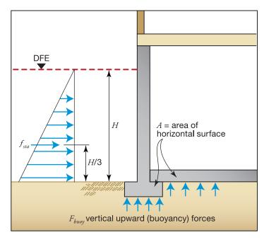
Figure 4-7. Diagram of hydrostatic forces
