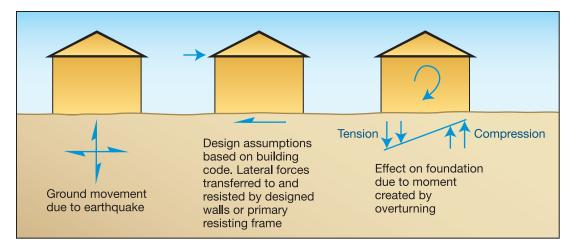
Figure 4-21. Seismic design causes and effects
