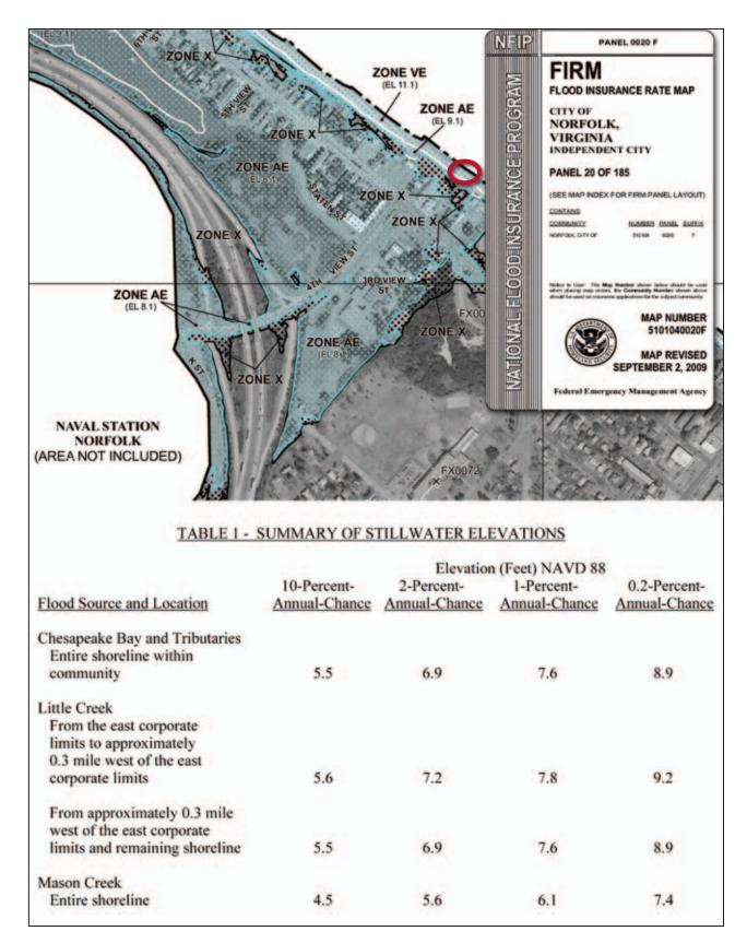
Figure 6-24. DFIRM excerpt and FIS excerpt: Summary of stillwater elevations for the Chester house
