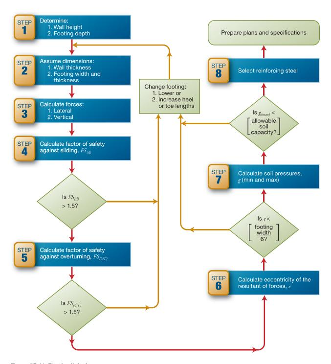
Figure 5F-11. Floodwall design process
