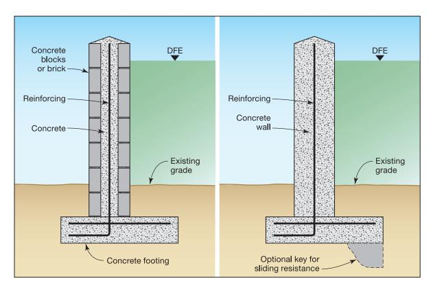
Figure 5F-6. Concrete cantilever floodwall reinforcement
