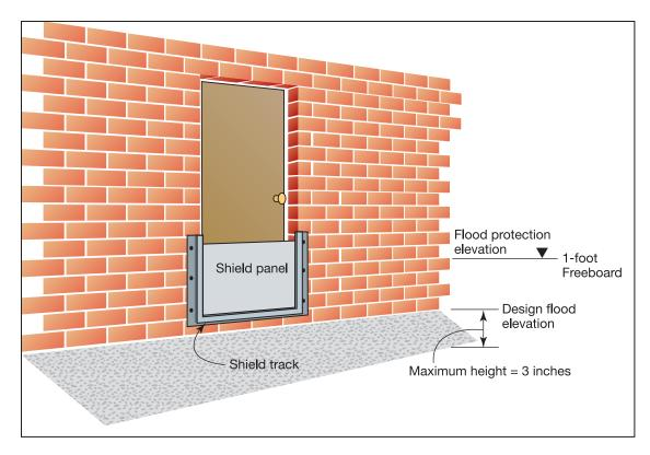
Figure 5D-5. A door opening may be closed using a variety of materials for shields.
