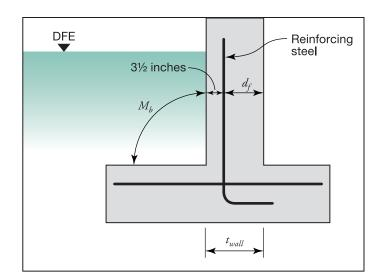
Figure 5F-16: Typical floodwall reinforcing steel configuration
