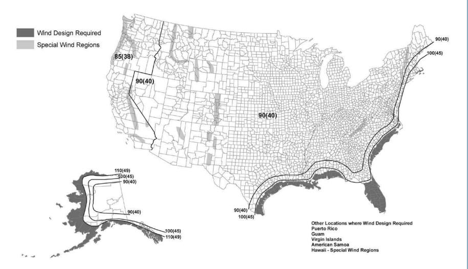
Figure 4-19B. Regions where wind design is required SOURCE: IRC, USED WITH PERMISSION
