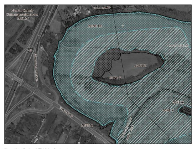
Figure 2-1. Typical DFIRM for riverine flooding
