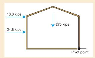
$\sum M_{pivot} = 0.7(13.3 \, \text{kips})(18 \, \text{ft}) + 0.7(24.8 \, \text{kips})(10 \, \text{ft}) - 0.6(275 \, \text{kips})(15 \, \text{ft}) = -2134 \, \text{kips} - \text{ft}$  OK, building weight keeps building from overturning.
