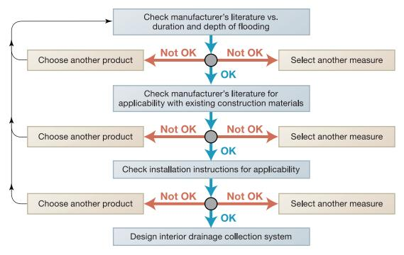
Figure 5D-17. Selection of sealants/coatings
