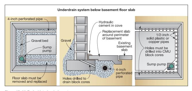
Figure 5D-27. Typical interior drain systems
