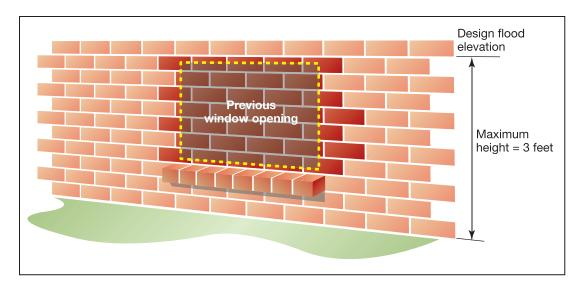
Figure 5D-7. Where a window is exposed to a flood, bricking up the opening could eliminate the hazard.
