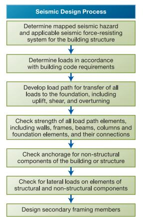
Figure 4-20. Seismic design process
