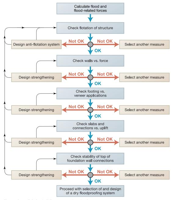
Figure 5D-10. Existing building structural evaluations
