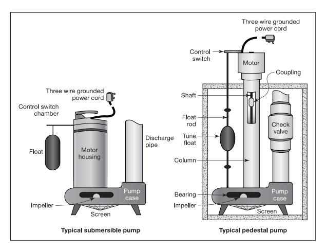
Figure 5D-28. Types of sump pumps
