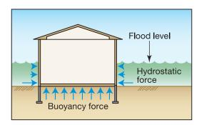
Figure 3-7. Hydrostatic and buoyancy forces
