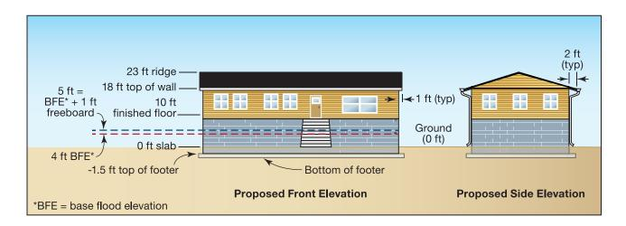
Extended foundation walls are proposed to be constructed of 8-inch-thick concrete masonry units. The existing footing is 2 feet wide by 1 foot thick concrete reinforced with (3) #4 rebar continuously. Top of footing is 18 inches below grade; soil type is stiff residual silts. New slab-on-grade will be 3½ to 4 inches thick and set at grade.
