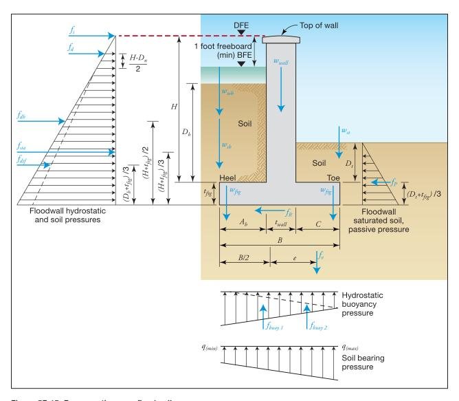
Figure 5F-15. Forces acting on a floodwall
