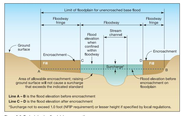
Figure 2-3. Typical riverine floodplain cross section
