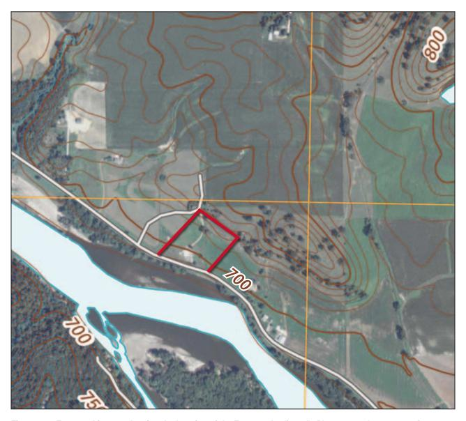
Figure 6-9. Topographic map showing the location of the Truman plot (in red). Please note these are 10-foot contours.
