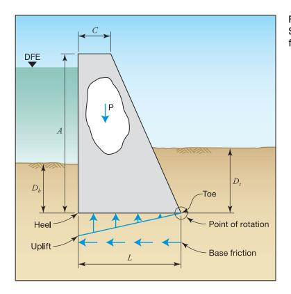
Figure 5F-5. Stability of gravity floodwalls
