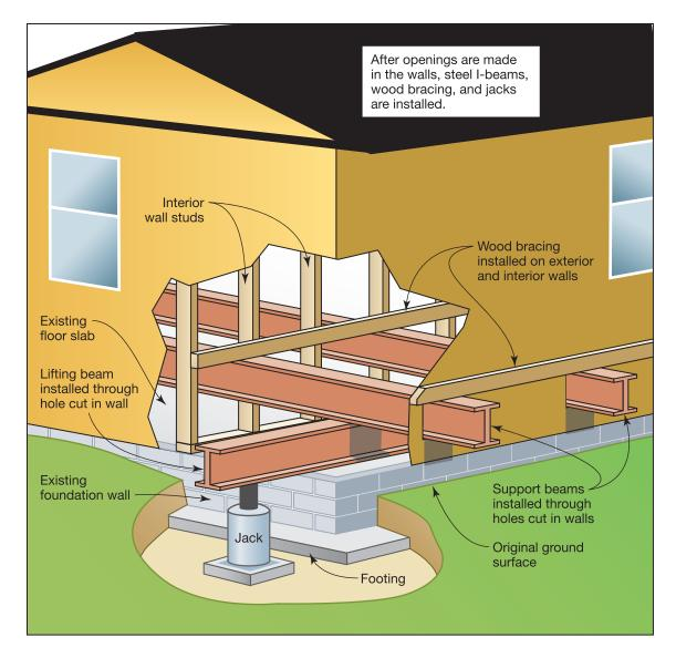
Figure 5E-17. Step 1 of elevating an existing wood-frame house without the slab using a new first floor constructed of wood trusses: Install steel I-beam network and prepare to lift walls
