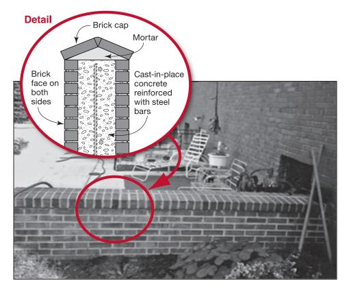
Figure 5F-1. Typical residential floodwall
