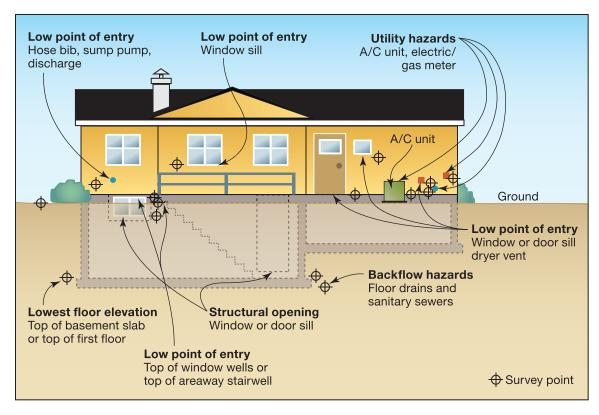
Figure 3-2. Survey to identify the low point of floodwater entry into a typical residential structure
