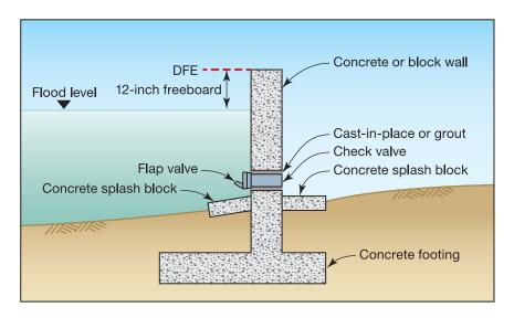
Figure 5F-22. Typical floodwall with check valve
