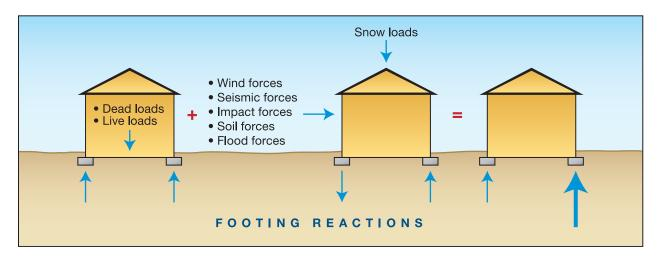
Figure 5-4. Foundation system loading
