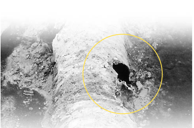
Corroded corrugated-metal outlet pipe removed from a dam that had developed large sinkhole.
