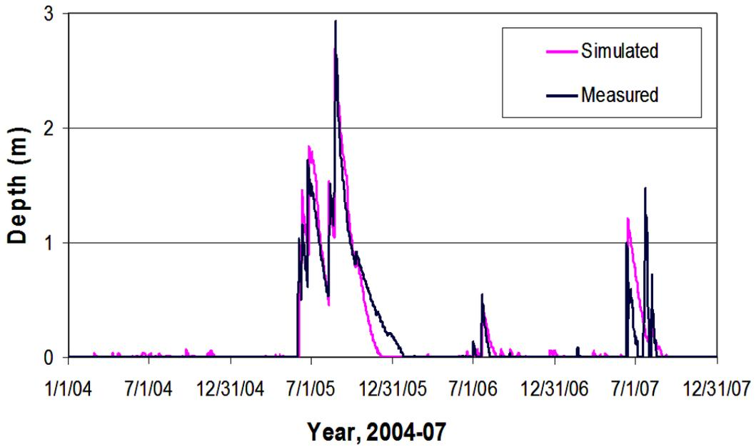
Figure 18. Simulated Versus Observed Water Depth Comparison for the DCN-Zimb Reservoir.
