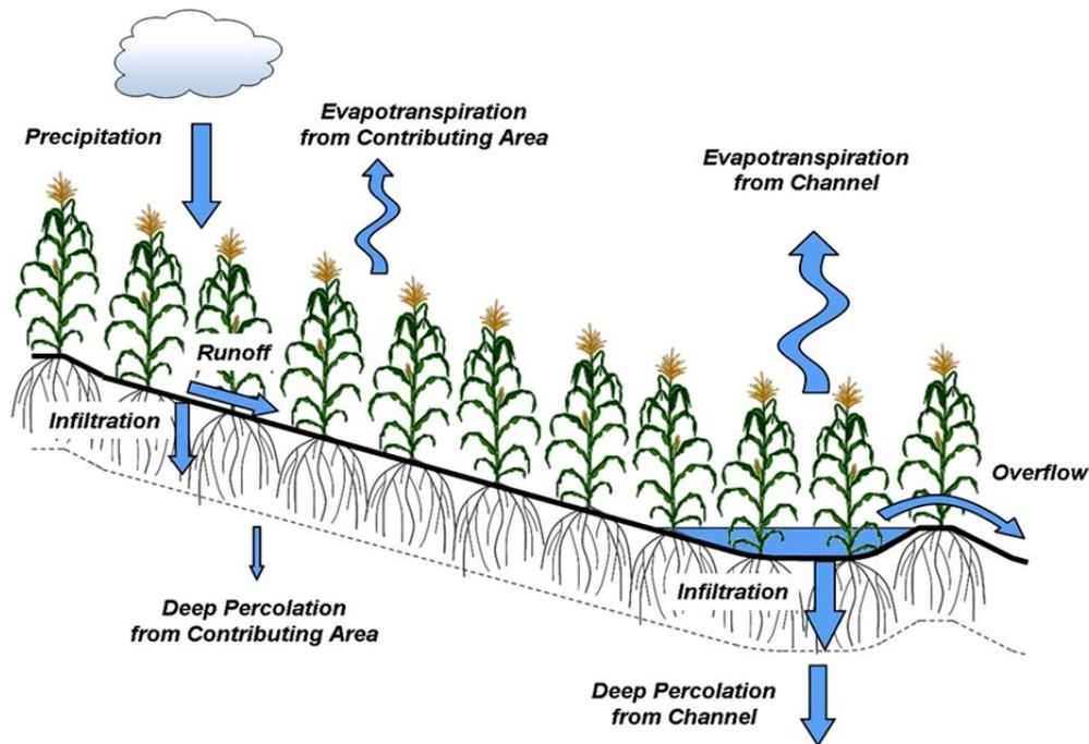
Figure 26. Water Balance Components of Terraced Land.
