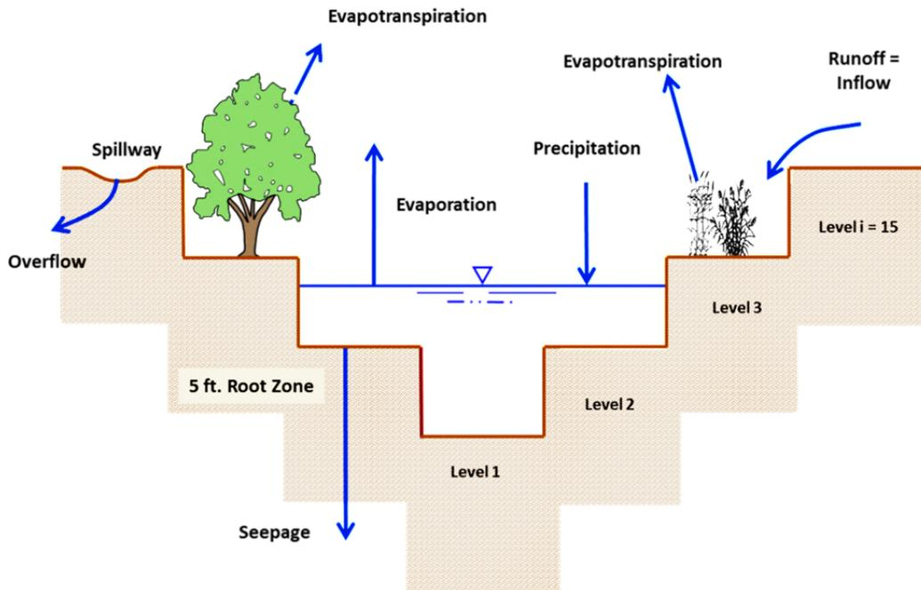
Figure 5. Reservoir Representation of Level Sections to Estimate Losses for Different Depths.
