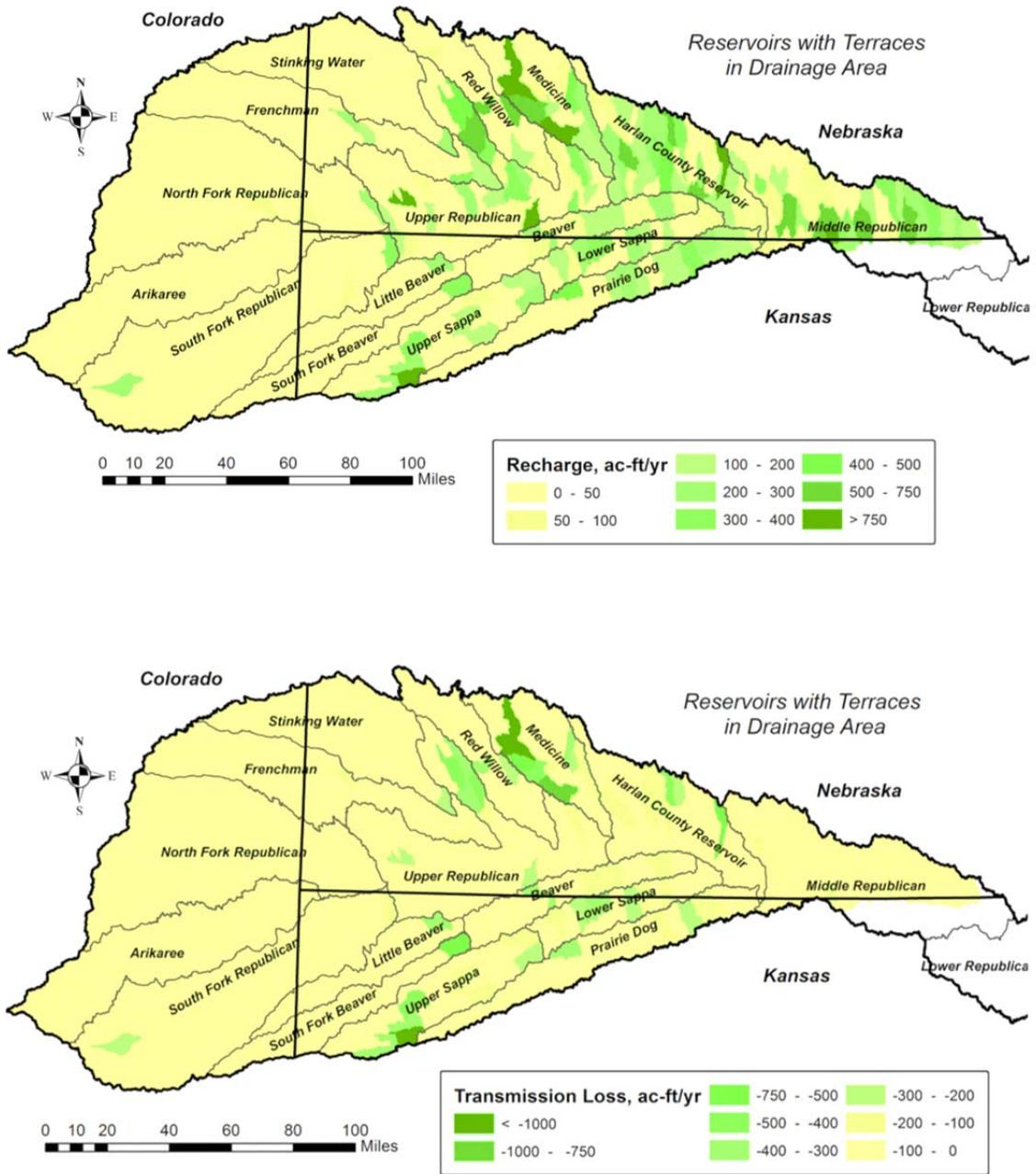
Figure 107. Distribution of Groundwater Recharge and Transmission Losses for the Scenario Considered the Effect of Reservoirs when Terraced Land is in the Drainage Area for the Reservoir
