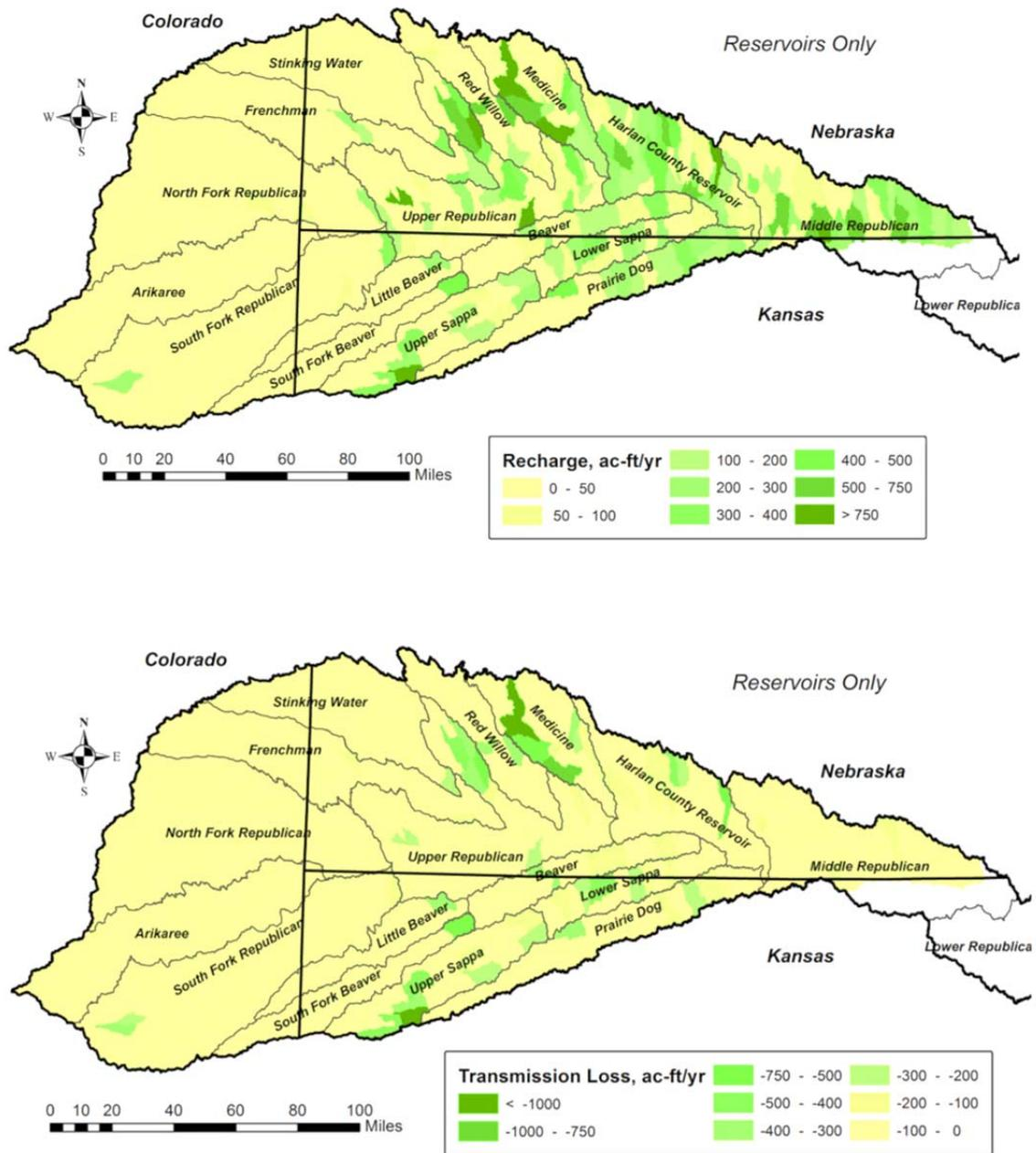
Figure 103. Distribution of Groundwater Recharge and Transmission Losses for the Scenario Considered only the Effect of Reservoirs
