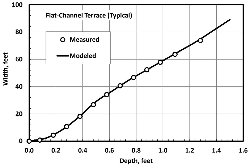
Figure 91. Depth-Width Relationship for a Typical Flat Cannel Terrace.
