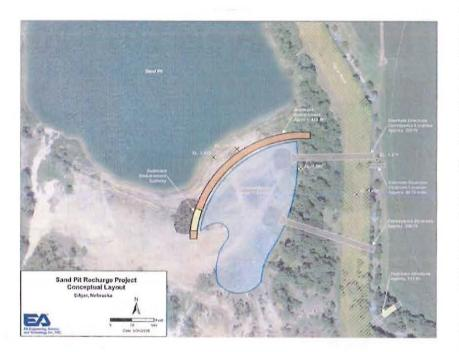
We are examining several projects which were identified for possible groundwater recharge and surface water quality improvement. One such project is a project which would capture excess surface water flows and drop them onto the fill sand section of an old gravel pit where it can be filtered before entering the water body of the pit, about 30 feet below channel grade. We have several areas where such applications might be possible. We are also working on
