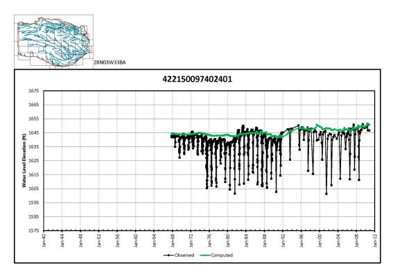
Graph 6e. Observed vs. Simulated Hydrograph for Well 422150097402401
