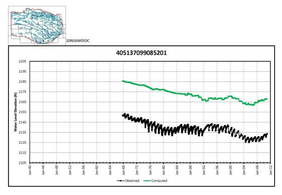
Graph 6f. Observed vs. Simulated Hydrograph for Well 405137099085201
