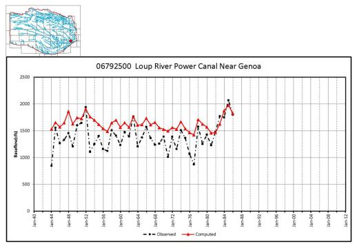
Graph 6k. Observed vs. Simulated Baseflow -- Loup River near Genoa. Data are from Loup River Near Genoa gage (06793000) adjusted by the Loup Power Canal diversions (gage 06792500).
