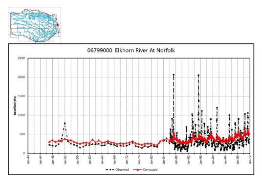
Graph 6i. Observed vs. Simulated Baseflow – Elkhorn River at Norfolk.
