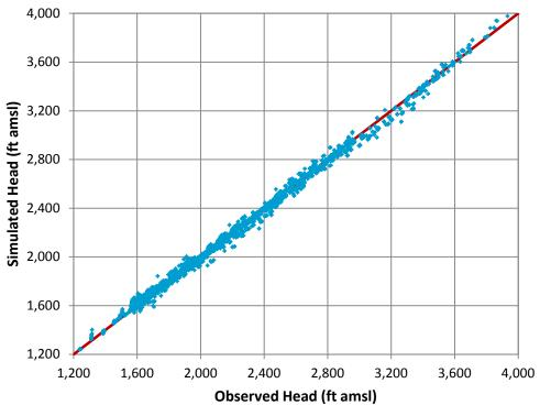
Graph 6a. Simulated versus Observed Head Targets
