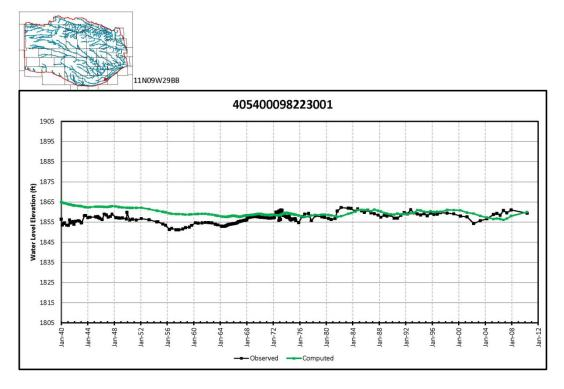
Graph 6d. Observed vs. Simulated Hydrograph for Well 405400098223001
