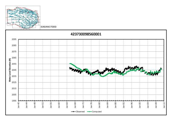
Graph 6c. Observed vs. Simulated Hydrograph for Well 4237300985600001
