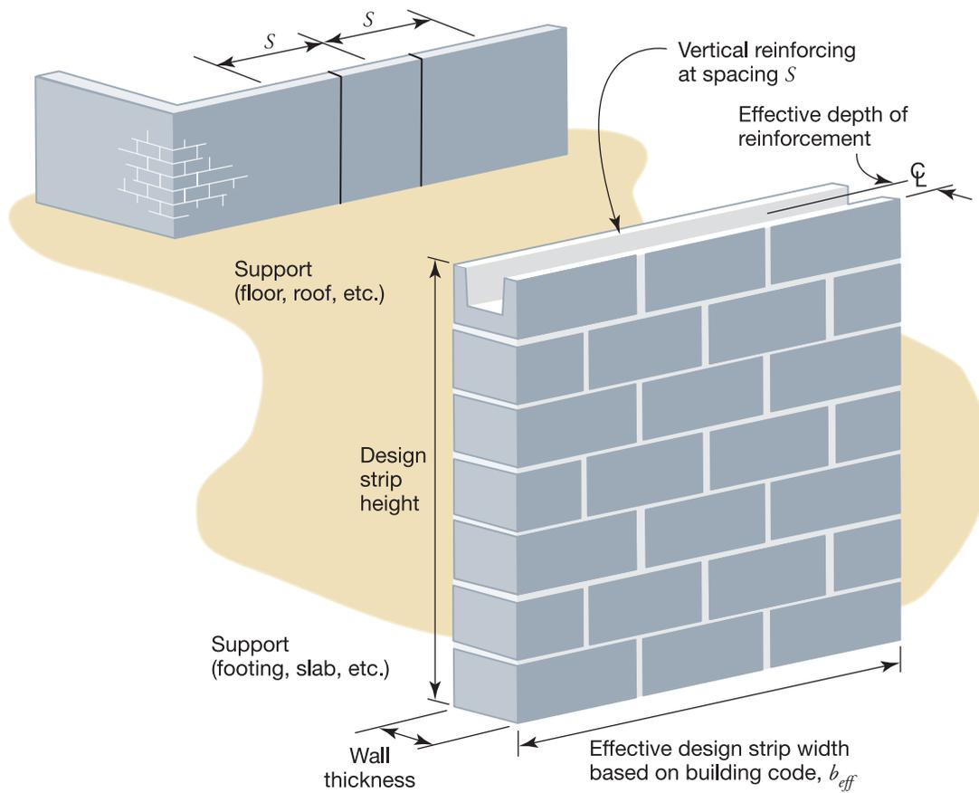
Figure 5D-13. Typical design strip for reinforced masonry
