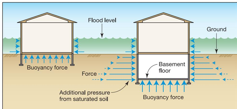
the designer wish to check the failure assumption, guidance is provided in Step 5. If floodwaters come into contact with a wood floor diaphragm (elevated floor or crawlspace home), the floor system/building superstructure should be checked for flotation (Figures 5D-11 and 5D-12).
