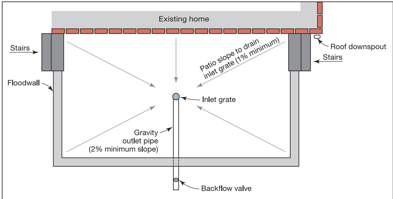
Figure 5F-19. Sample patio drainage to an outlet
