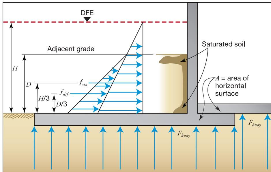
Figure 4-8. Combination soil/water hydrostatic and buoyancy forces
