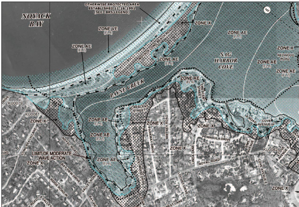
Figure 2-2. Typical DFIRM for coastal flooding showing the Limit of Moderate Wave Action (LimMW)
