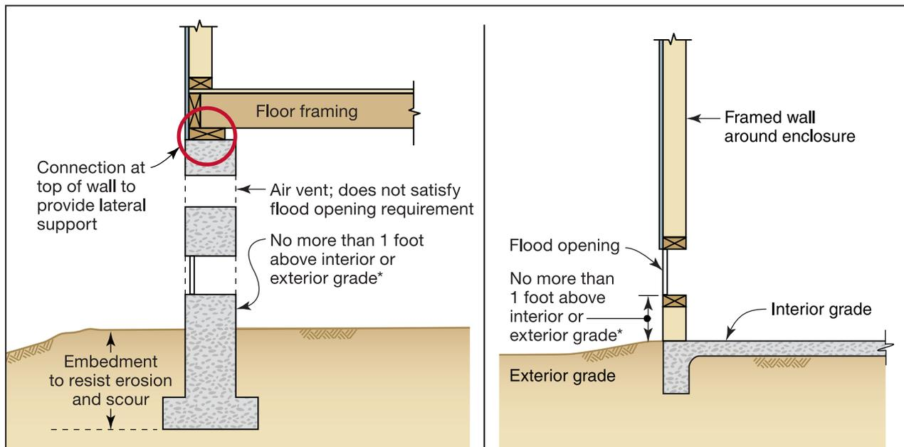
Figure 5E-13. Typical opening for solid foundation wall
