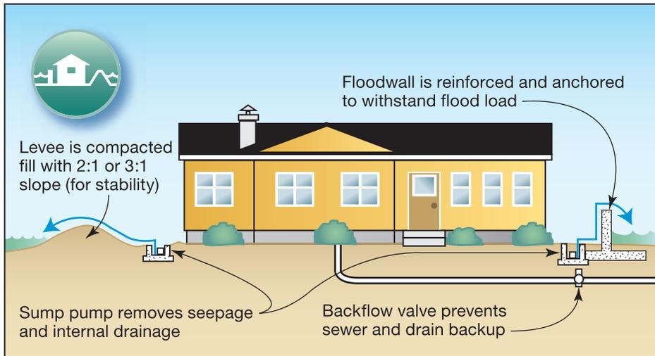
Figure 1-11. Structure protected by floodwall and levee
