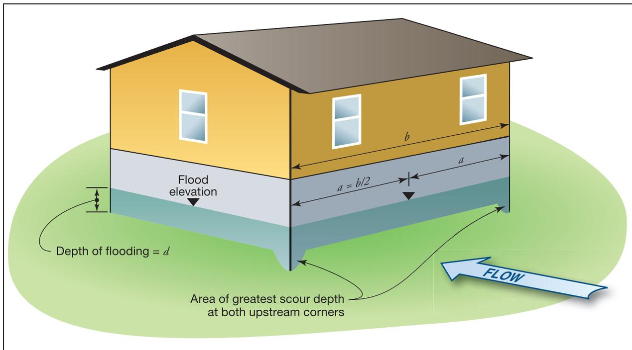
Figure 4-24. Scour action on a ground level building
