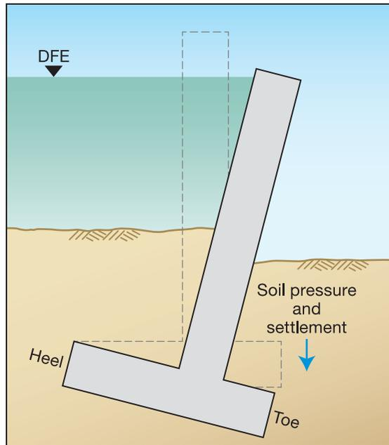
Figure 5F-14. Failure due to excessive soil pressure
