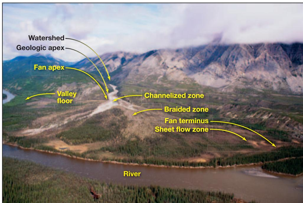
**Sheet Flow Zone:** Downstream of the braided zone characterized by flow depths less than ½ foot (flow depths normally decrease in the downfan direction). Smaller channels may aggrade while other areas are subject to erosion or scour. Flow may continue to spread laterally until sheet flow is predominant. Floods are usually limited to inundation by low velocity floodwater.
