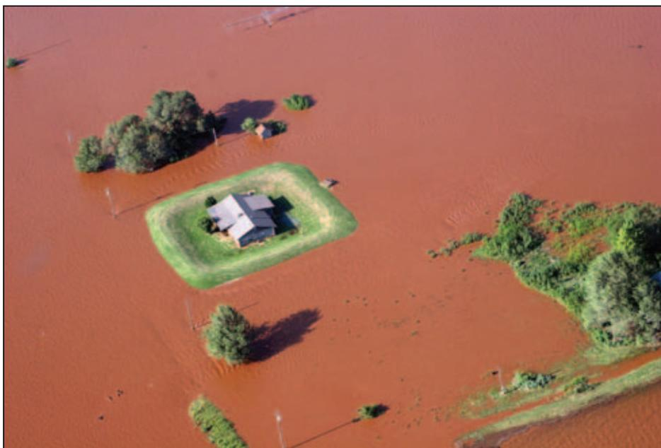
Figure 1-12. Home protected by a levee
