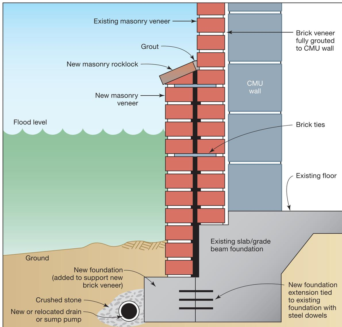
**Figure 5D-2.** A way to seal an existing brick-faced wall is to add an additional layer of brick with a seal in between. Please note that weep holes and wick drains work both ways to allow for moisture passage from high to low pressure. Weepholes and flashing should be located above the DFE, and the veneer below the DFE should be fully grouted.
