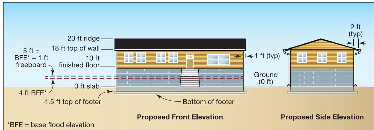
Extended foundation walls are proposed to be constructed of 8-inch-thick concrete masonry units. The existing footing is 2 feet wide by 1 foot thick concrete reinforced with (3) #4 rebar continuously. Top of footing is 18 inches below grade; soil type is stiff residual silts. New slab-on-grade will be 3½ to 4 inches thick and set at grade.
