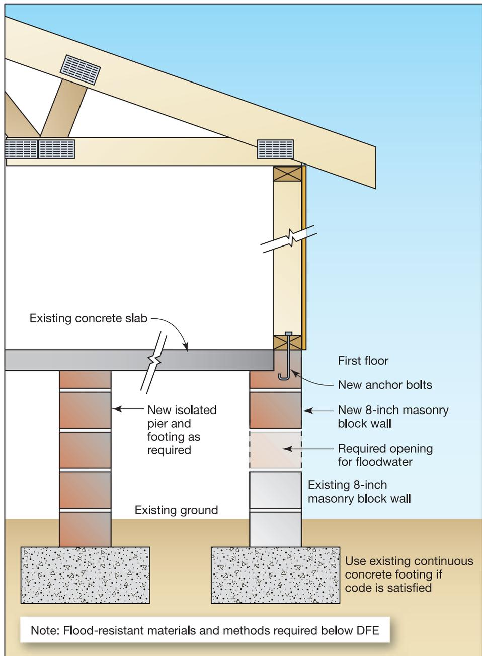
The entire elevation design process is illustrated with a detailed example of the design for a crawlspace house (Figure 5E-24).
